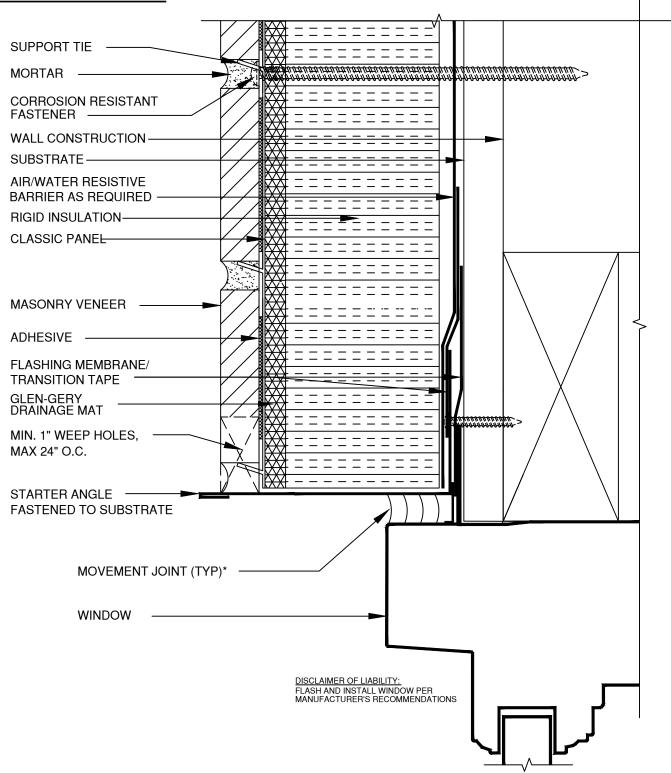
RECESSED WINDOW HEAD WITH INSULATION DETAIL (ALTERNATE)
