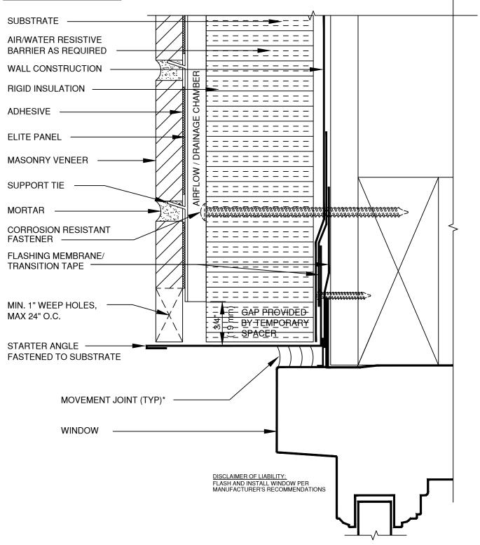
RECESSED WINDOW HEAD WITH INSULATION DETAIL (ALTERNATE)
