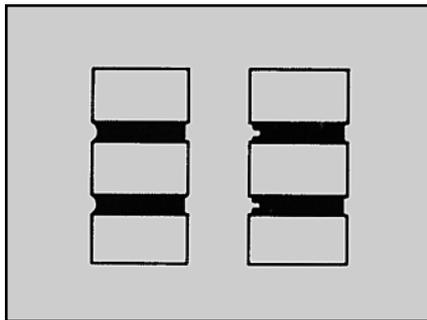
mortar and units. Do not use struck or raked joints in exterior brick masonry. The most important factor in the construction of dry masonry walls is the proper filling of the mortar joints. Poorly filled joints result in voids and separation cracks through which water may enter, particularly when there are wind-driven rains. Bed joints must be solid
