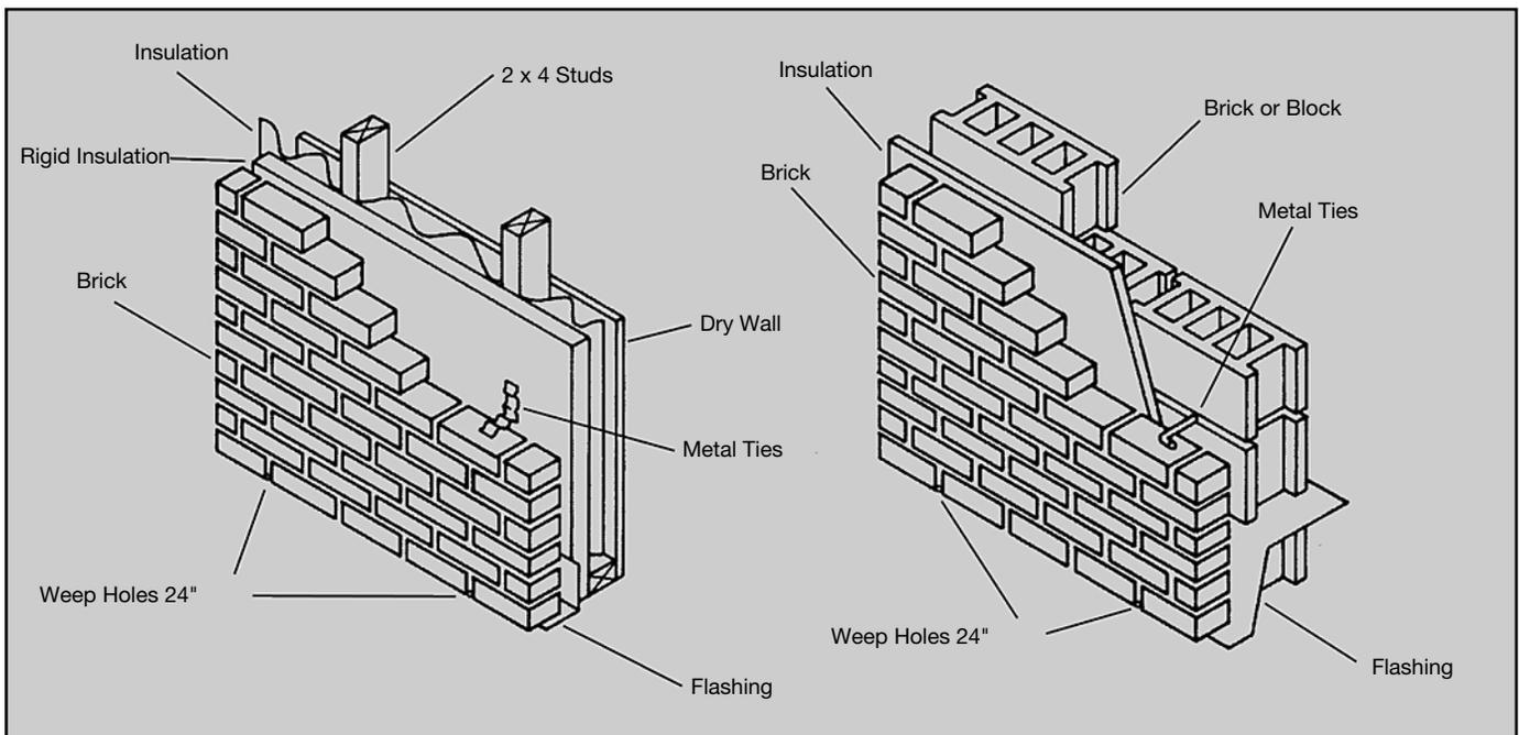
flashings be held back from the face of the wall about one-half inch. Do not do this! Water can run around the end of the flashing and back into the wall. Instead, either extend the flashing beyond the face of the wall and then cut it flush or use small stainless steel flashing extensions for the exposed portions of the flashing. Through-wall flashings should be used:
