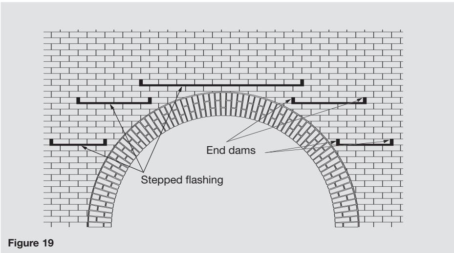
flashings laid in or attached to the back-up which then drop down at least eight inches, run horizontally, and then pass through or under the brick wythe to the outside.
